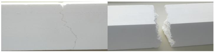
An example of the extra toughness PATI delivers is evident in the image above left. Bars used in 3-point bend (MOR) test break but do not separate as does other non-reinforced, rigid-fiber insulation as shown above right.
