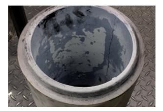
Shown in the image to the left is a PATI cylinder after being removed from the 1600°C (2912°F) hightemperature thermal process system it is used in. Unique to PATI is its ability to remain intact dispite exhibiting typical thermal shock cracks. PATI's reinforcement enabled this cylinder to be used for many cycles, removed from the system intact, reinstalled with other new components and reused for many more cycles. The end result is lower cost of ownership.
