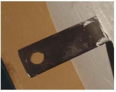
accomodate the current draw of each custom-made RDI heating element. Strip sizes range from 1mm(0.04") to 3mm(1.3") thick x 12.5mm(0.5") to 25mm(1.0") wide.
