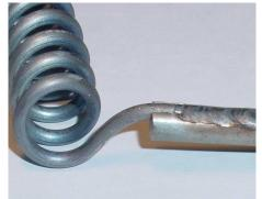
Solid rod leads with or without threaded Easily bolted, strip leads are sized to ends are securely mig-welded to the FeCrAl resistance wire. Welded leads are stress-annealled before the RDI heating element assembly is vacuumformed.
