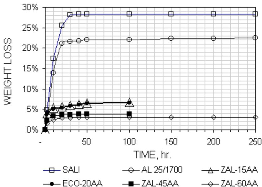
Weight Loss results for alumina bonded types tested.
