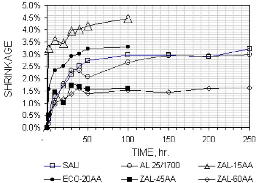
Shrinkage results in thickness directions for all types tested.
