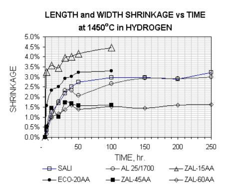
Shrinkage results in thickness directions for all types tested.
