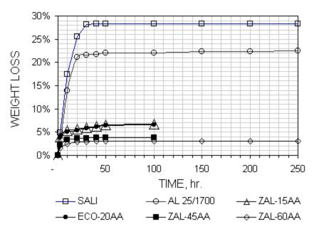
WEIGHT LOSS vs TIME at 1450°C in HYDROGEN
