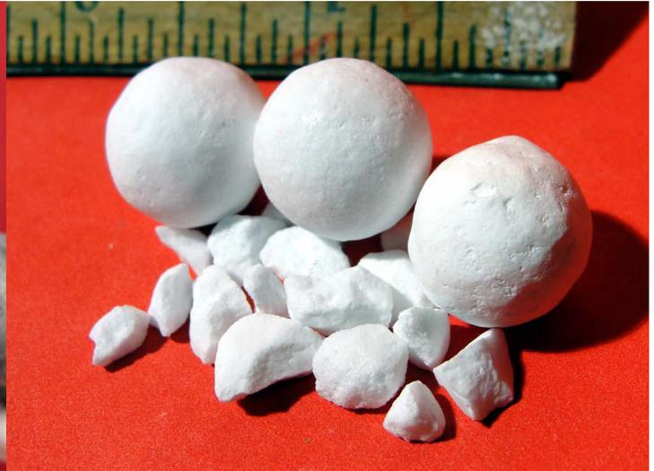
**Tabular Alumina Filter Balls and Gravel** for deep bed filtration systems. High density and fired at high temperatures, ZCI's Tabular Alumina Filter media play a very important role in enhancing the value of each ton of cast metal.
