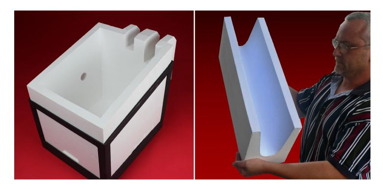
These images above show a Uniform A-1 "Head Box" (left) and a "Trough" (right) which are parts of molten metal delivery systems on Twin Roll Aluminum Sheet Casters. UA-1 with a surface treatment of colloidal silica followed by top coat of SLICOAT ES Boron Nitride can deliver high-quality clean metal ton after ton after ton.
