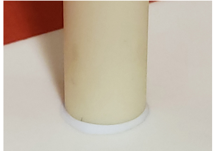
DB1 can be used to bond fine grained dense Al_2O_3 together, as shown above.
